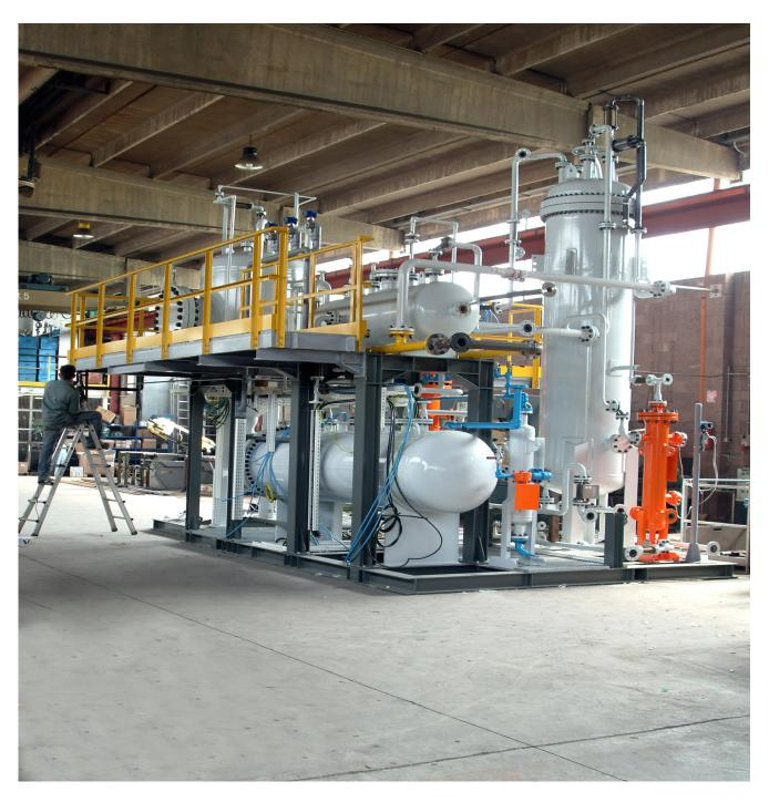
BEA Technologies designs amd manufactures fully automated AMINE filtration packages for the removal of solid contaminants, cook fines, acid condensates from the amine solution circulating in gas sweetening plants. The filtration of amine solution serve to protect internal critical parts of re-boilers and injectors from corrosion damages.
